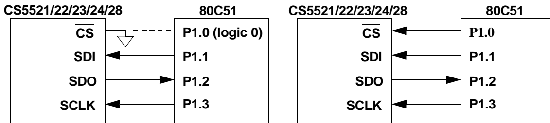
Figure 1. 3-Wire and 4-Wire Interfaces
