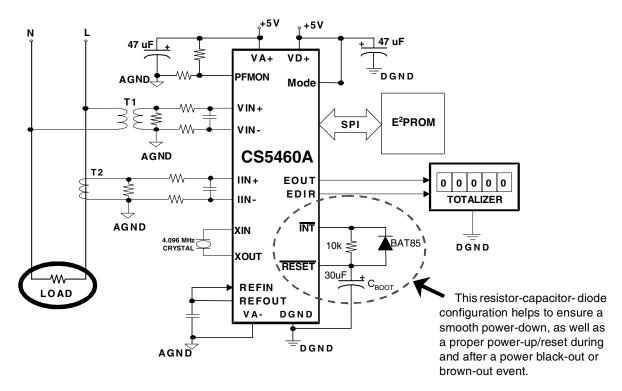
Figure 1. CS5460A Auto-Boot Configuration: Automatic Restart After Power Failure
