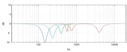
7-band equalizer characteristics after calibration.
