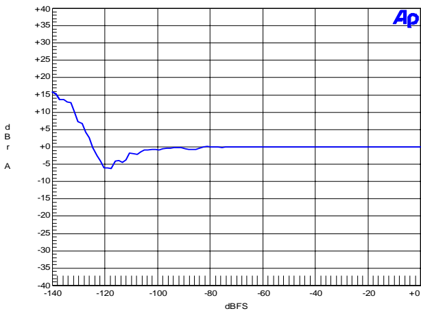
Figure 27. 192 kHz, Fade-to-Noise Linearity
